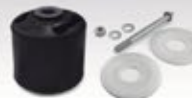
• FM-B922610 Suspensiones HLM, HLM-1, HLM-1-T KIT BUJE TRI-FUNCIONAL ALINEACION RAPIDA HENDRICKSON | S24691 GAFF | 13628
